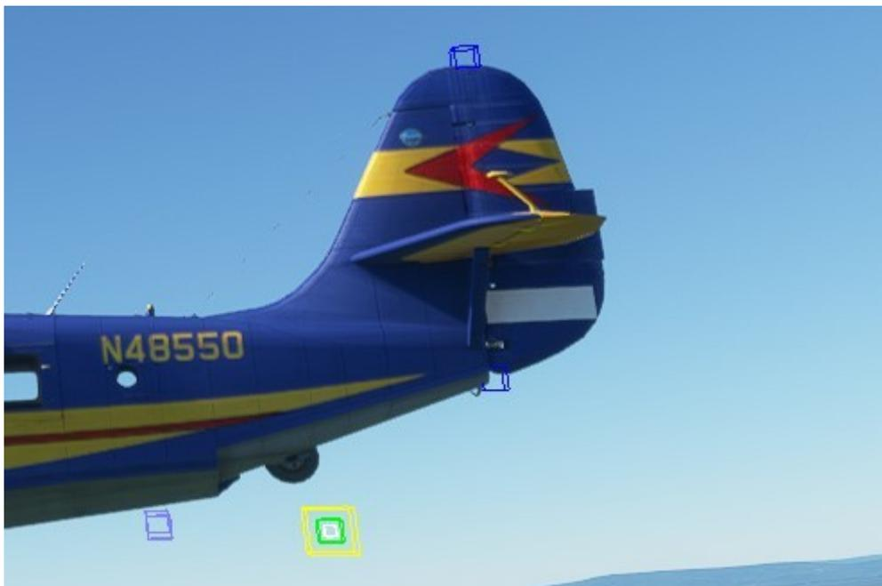
The vtail\_pos\_vert is between the blue box at the top of the vtail and the blue box at the bottom of the vtail. The blue box is a [CONTACT\_POINTS] point.X class 2.
